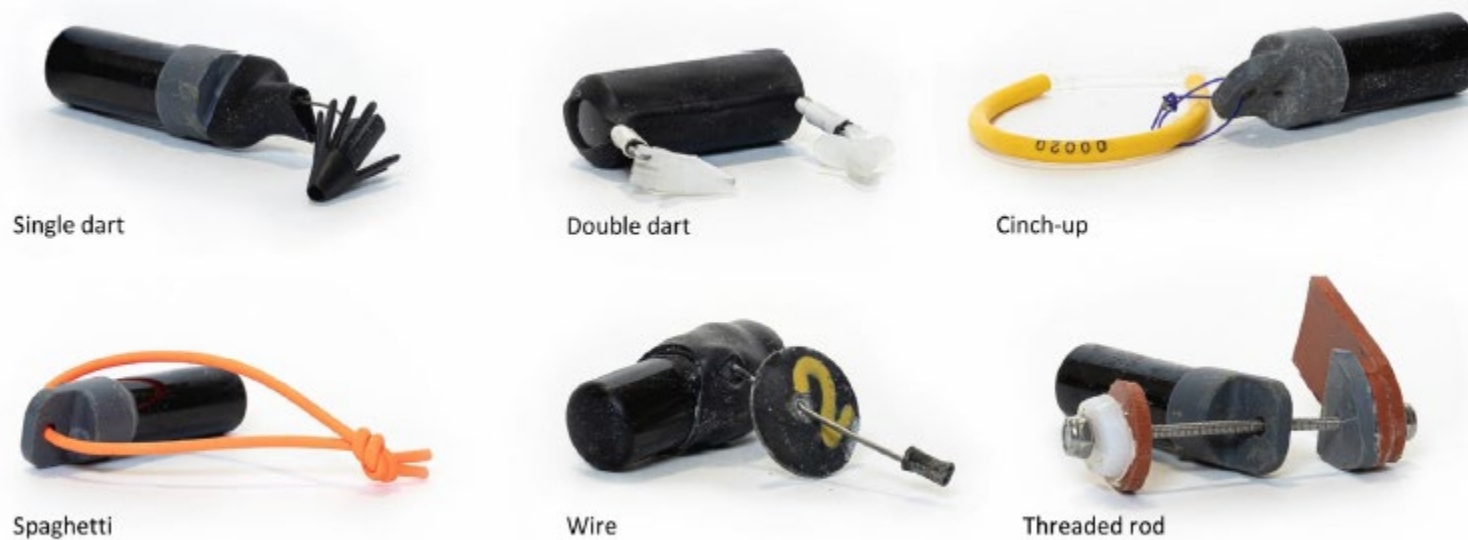
FIGURE 1 Six methods for attaching acoustic transmitters to fish
